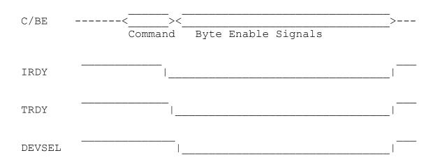
PCI transfer cycle, 4 data phases, no wait states. Data is transferred on the rising edge of CLK.
