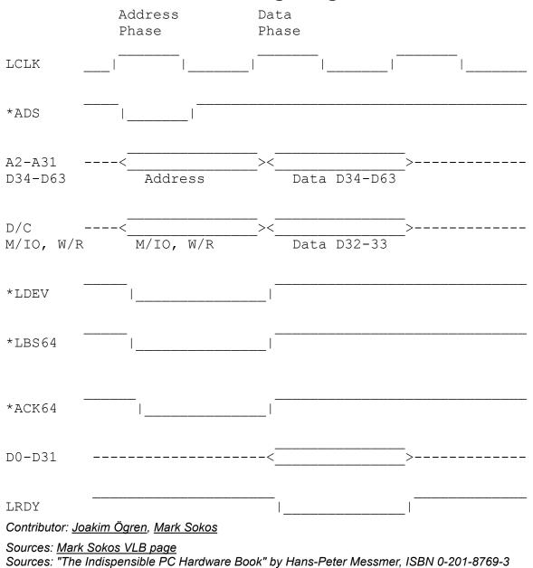
64 Bit Data Transfer Timing Diagram:
